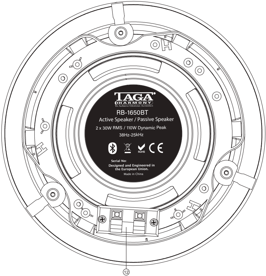
12. MASTER SPEAKER INPUT terminal - Spring Clips [+ and -]
