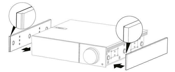
When installing new magnetic side panels, please ensure that the groove cuts are aligned with the direction of the front panel. Insert from the rear by holding the rear of the panel.
