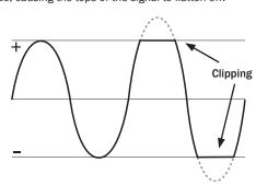
When the 851W detects clipping this LED will briefly flash. If the clipping reaches a dangerous amount that could damage the amplifier or attached speakers the unit will then go into protection.
