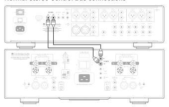
When using the 851W in either Bi-amped dual mono connection or in Bridged dual mono connection the following Control Bus connections must be made.
